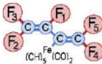
FIG. 2: Custom-designed Fluorine molecule used as a quantum computer to solve a simple problem (courtesy IBM Research).
