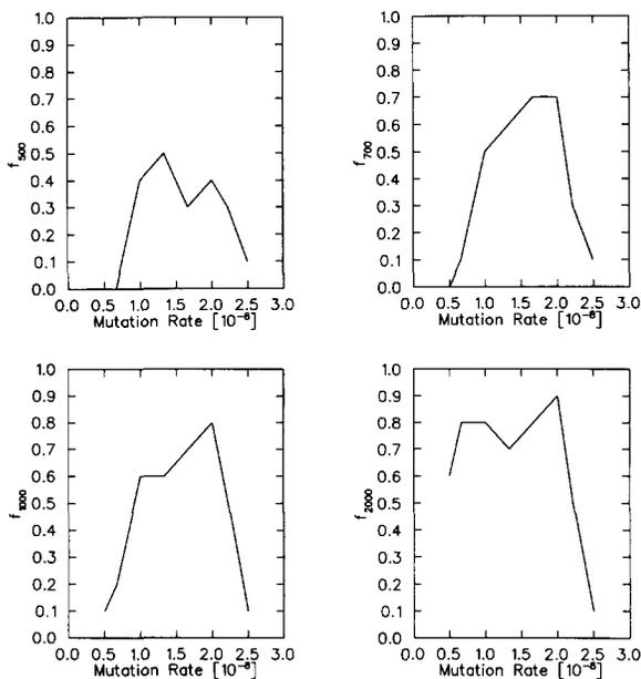
Fig. 5. Learning fractions  $f_X$  as defined in the text versus mutation rate for various cutoffs. (a) Cutoff  $X = 500$  million instructions, (b)  $X = 700$ , (c)  $X = 1000$ , and (d)  $X = 2000$ .
